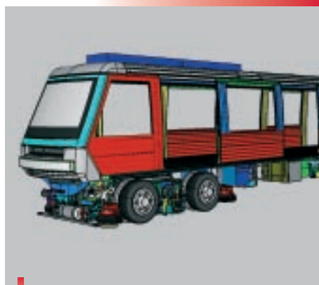
Our motorized bogies with rubber tires are the best solution for Lausanne's record gradient of 12%.
